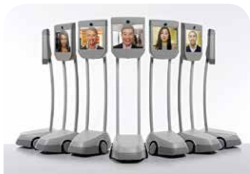
Called simply "Beam," the Smart Presence System is your remote physical presence that can be driven around to interact with people.
